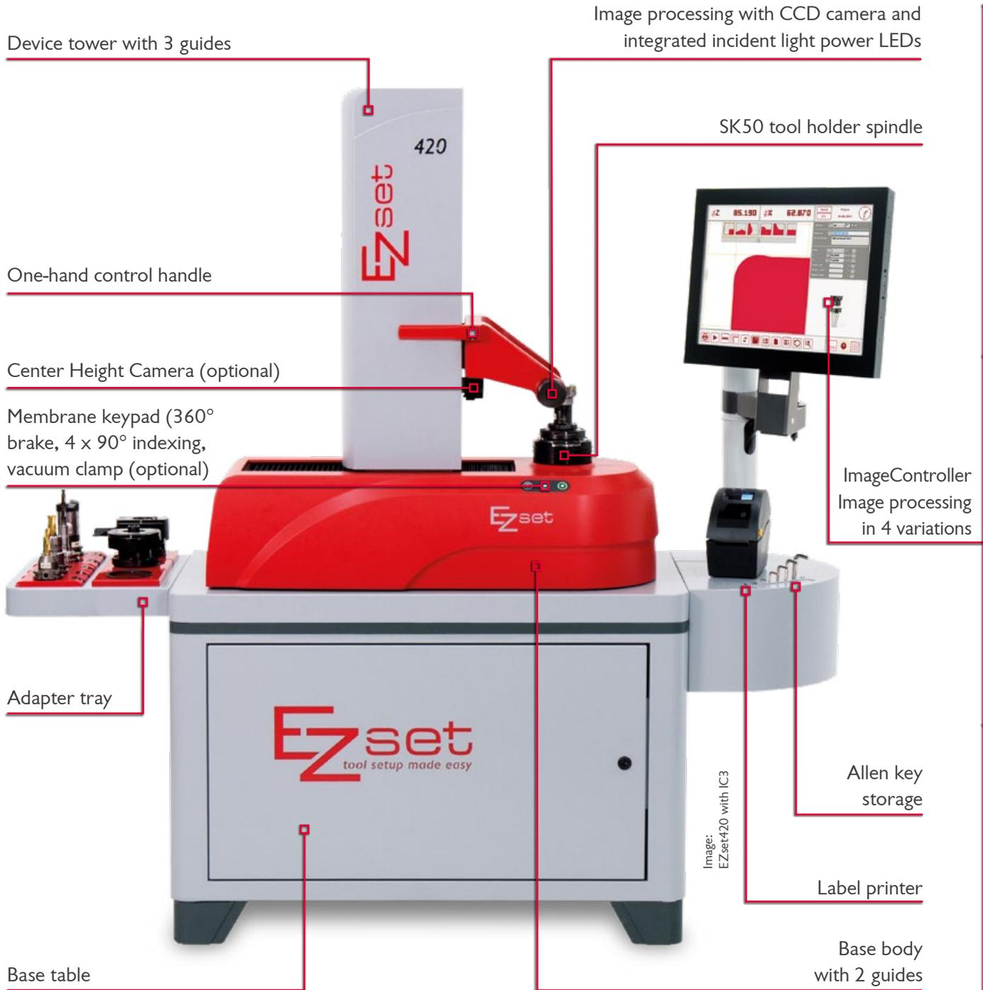
EZset tool presetters are available with a variety of measurement ranges, and with the four image processing variations ICbasic, IC1, IC2, and IC3.
